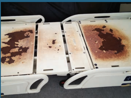
RUSTED BED DECK
