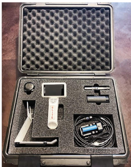
Healthmark EPRO-001SK (EndoPro-Cam) is used to identify damage to the optics in rigid endoscopes
