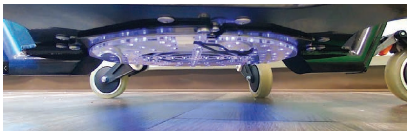
Finsten Technologies' THOR UVC Halo disinfects the floor and its own wheels.
