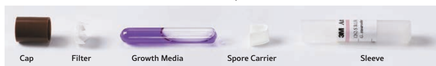
FIGURE 1 – Components of a self-contained rapid readout biological indicator.
