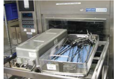
Figure 2- Improper loading of instruments (with silicone mat in bottom of tray).
