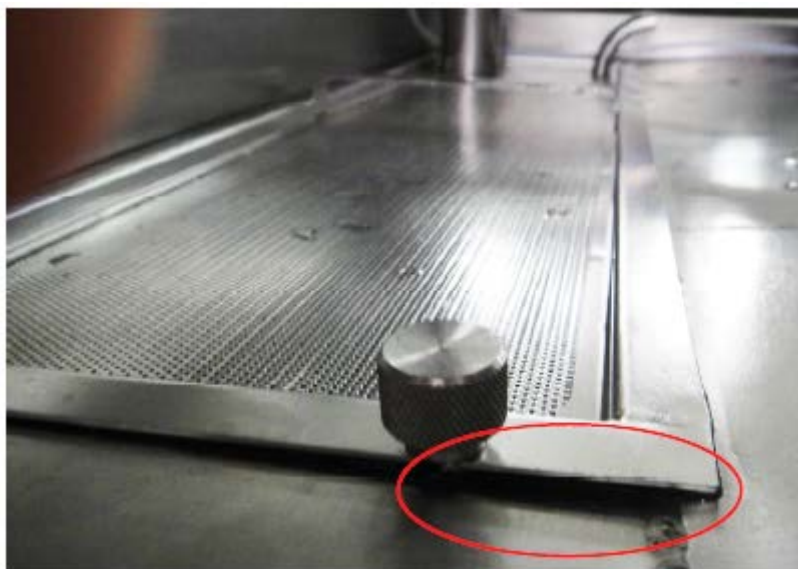
Figure 4: Washer debris screen installed incorrectly.
