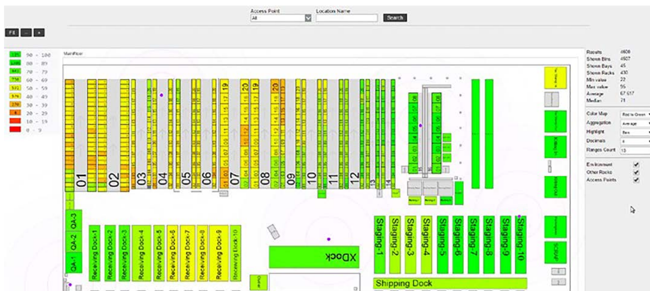
Figure 1 – Slotting analytic with 2-D warehouse mapping from Generix Group
