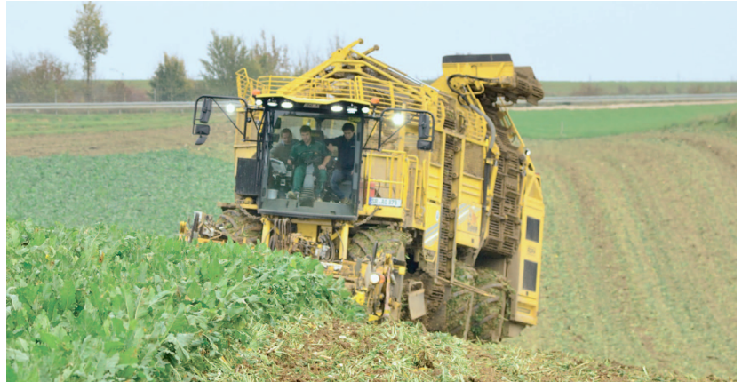
This harvester's hydraulic chassis system features an oscillating front axle and two rear axles with hydraulic suspension to reduce sway and increase stability on grades.
