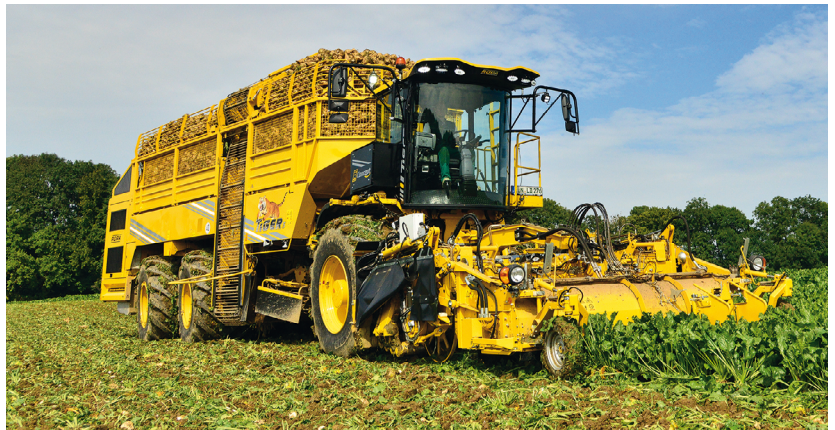
Two adjustable motors and a constant-speed motor work together to help this harvester achieve maximum traction force without losses.
