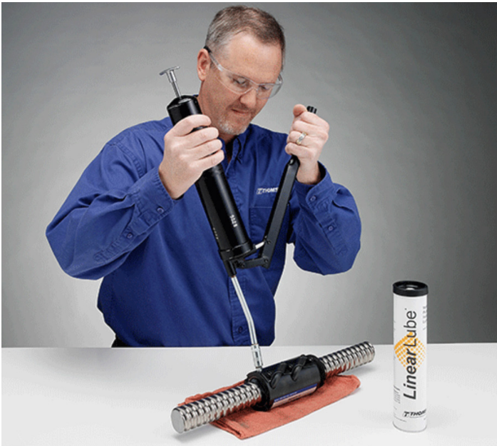
The author, Jeff Johnson, uses the correct lubrication method to apply Thomson's™ Linear Lube to a ball screw.
