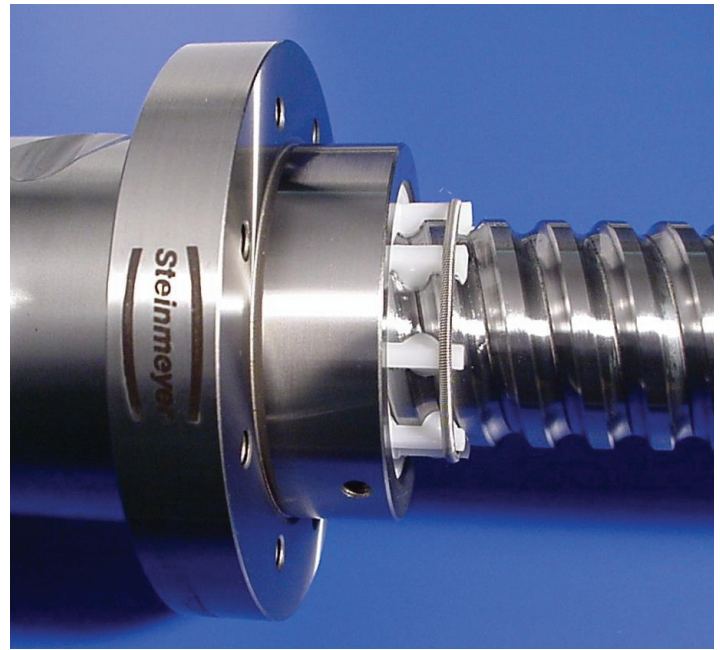
Plastic wiper “fingers” should precisely fit into the surface of the screw thread to clean them prior to passing through the ball screw. Note the spring used to preload or tension them against the screw threads.
