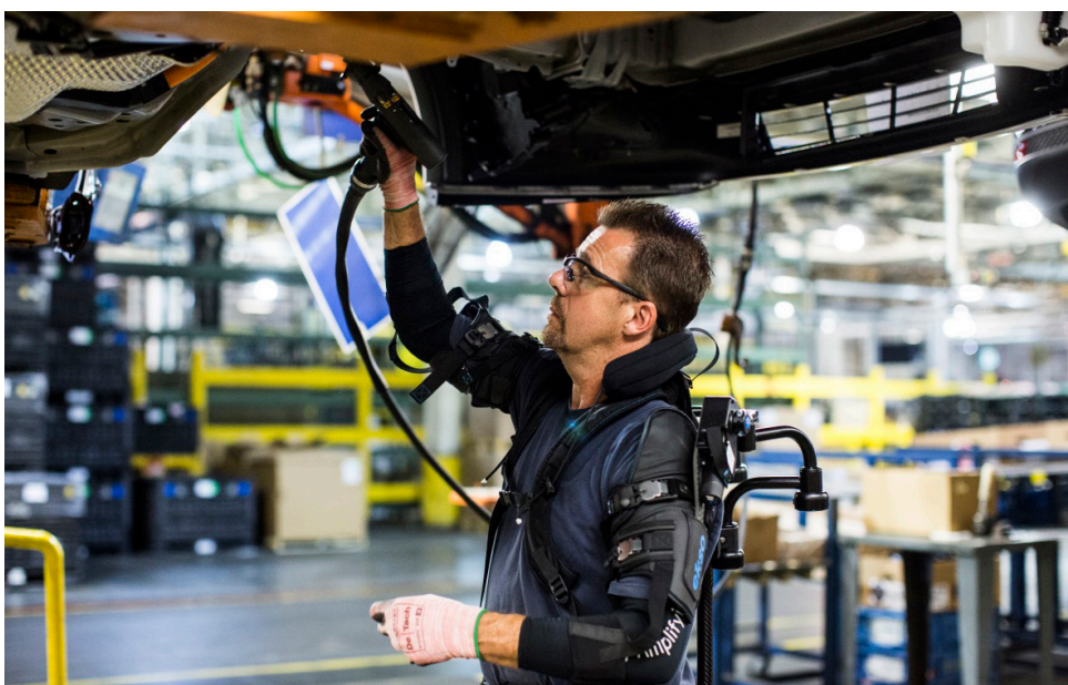
The EksoVest is an upper body exoskeleton that elevates and supports a worker’s arms to assist them with tasks ranging from chest height to overhead.
