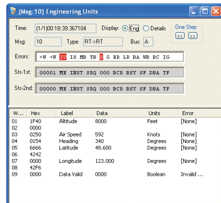
Figure 8 All BusTools analyzers simplify traffic analysis by allowing traffic to be displayed in engineering units.
