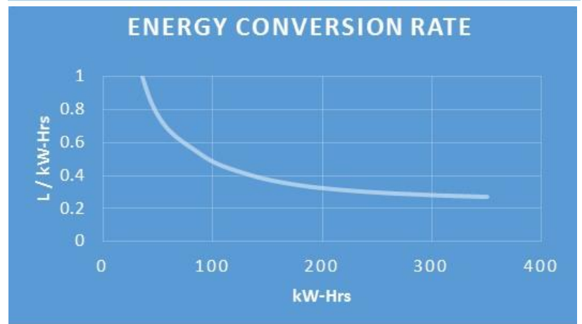
Electrical energy conversion from diesel fuel
