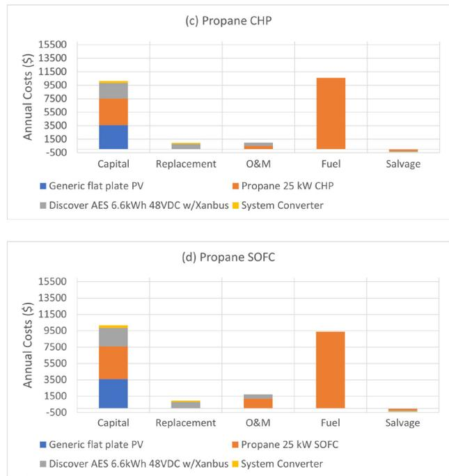
Figure 1: Unincentivized annualized costs for the hybrid microgrid with a) Diesel generator b) Propane COTS, c) Propane CHP and d) Propane SOFC generation systems.
