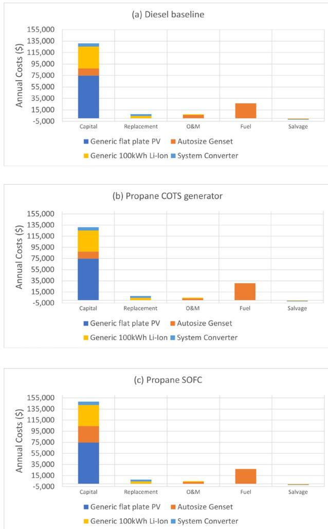
Figure 5: Unincitvized annualized costs for the hybrid microgrid with a) Diesel generator b) Propane COTS generator, and c) Propane SOFC generation systems.
