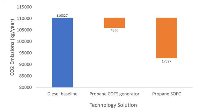
Figure 7: Tailpipe CO<sub>2</sub> emissions for different generation systems.
