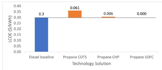
Figure 2: Unincentivized LCOE of the hybrid microgrid system with different generation systems.
