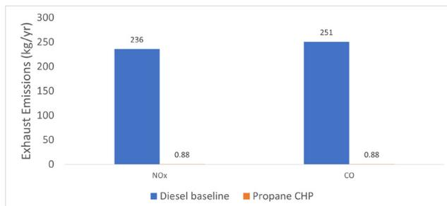
Figure 4: NO<sub>x</sub> and CO emissions for the baseline diesel and propane CHP generation systems.
