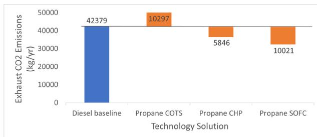
Figure 3: Tailpipe CO<sub>2</sub> emissions of the four generation systems.
