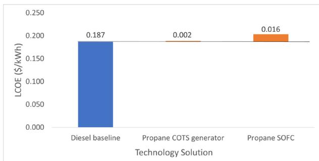
Figure 6: Unincitvized LCOE of the hybrid microgrid system with different generation systems.
