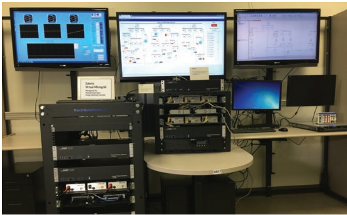
Figure 6: Eaton's virtual microgrid managed by the physical Power Xpert Energy Optimizer™ controller
