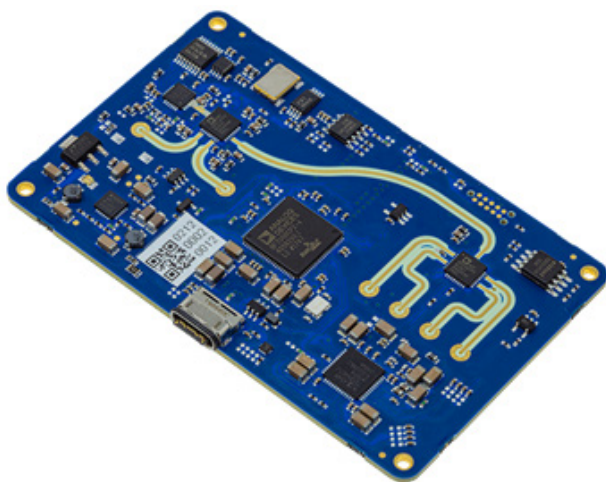
3. For ease of evaluation, separate 24-GHz transmit and receive ICs are mounted on a compact model EV-TINYRAD24G PCB. (Courtesy of Analog Devices).
