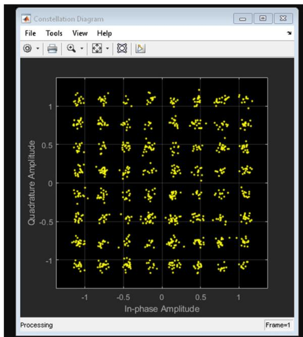
**3. 1024QAM is one of the features implemented in Wi-Fi 6 for increased data speed and capacity. This diagram shows a QAM constellation diagram with 64 symbols. (Courtesy of MathWorks)**
