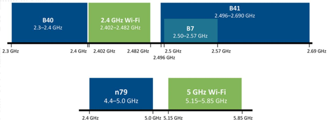
1. The 2.4-GHz Wi-Fi channel is adjacent to the n41, n40, and n7 spectrum, while the n79 band is adjacent to the 5-GHz Wi-Fi channel.
