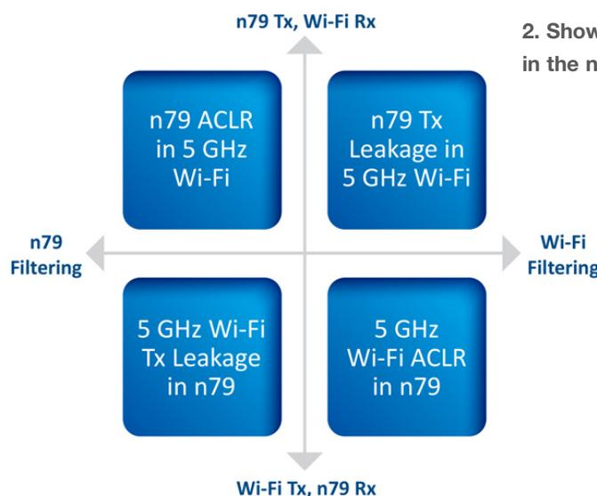
2. Shown is a simple illustration of interferences in the n79 and Wi-Fi coexistence cases.
