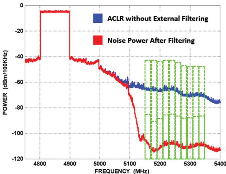
5. This plot demonstrates high-rejection filtering with an n77/79 antennaplexer (not to scale).
