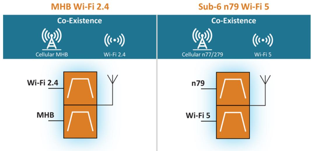
6. Antennaplexers enable happy coexistence for 2.4-GHz Wi-Fi and 5-GHz Wi-Fi.
