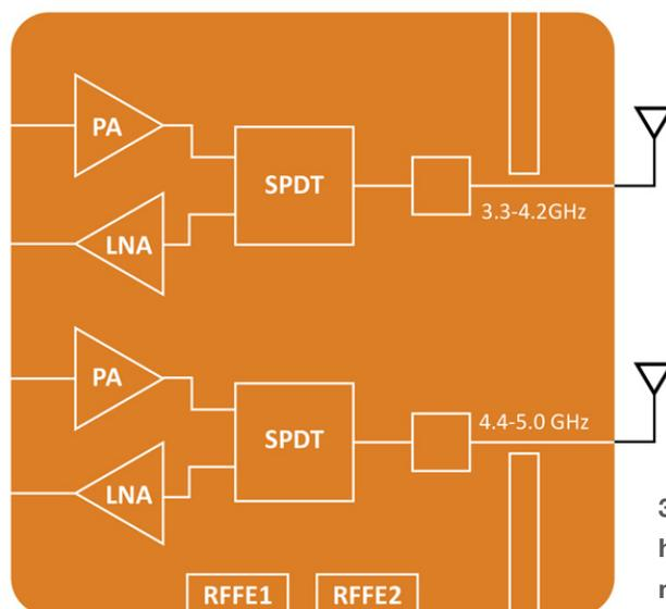
3. Skyworks' SKY58255 module is an ultra-high band Tx/Rx module supporting bands n77 to n79.
