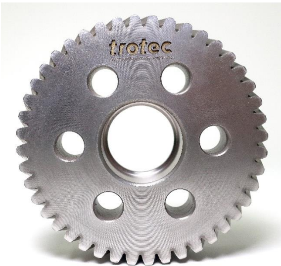
Deep engraving of a logo on a steel gear
