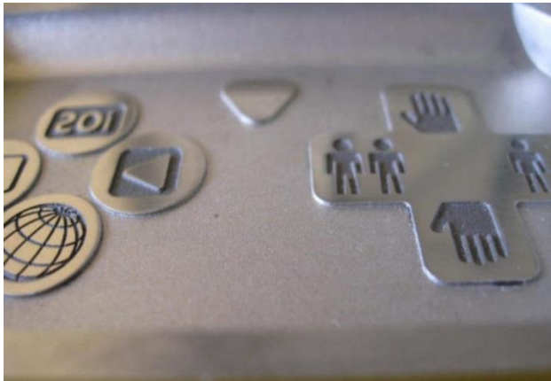
Deep engraving on stainless steel control pad
