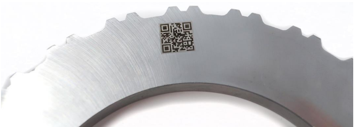
QR code engraved on stainless steel part for asset tracking
