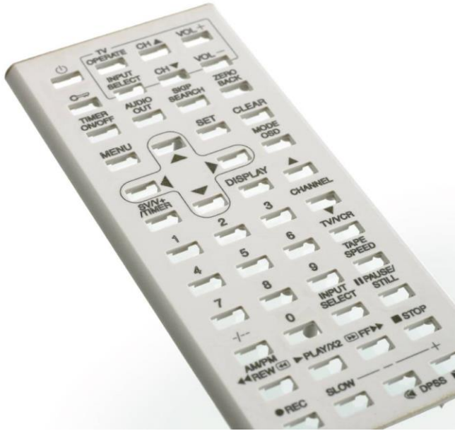
Small lettering laser marked on remote control using the color change method
