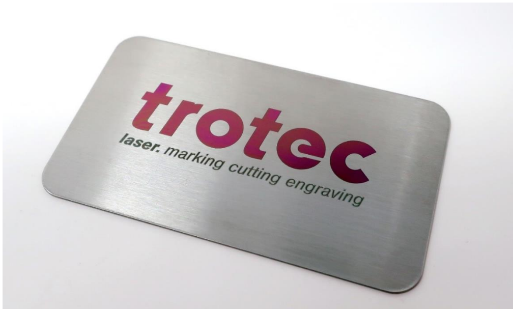
Logo marked on stainless steel plate with the metal color change process.
