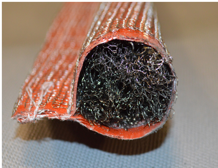
Figure 4. Tadpole Gasket constructed of stainless steel mesh, silicone coated cover with stainless steel mesh overlay.
