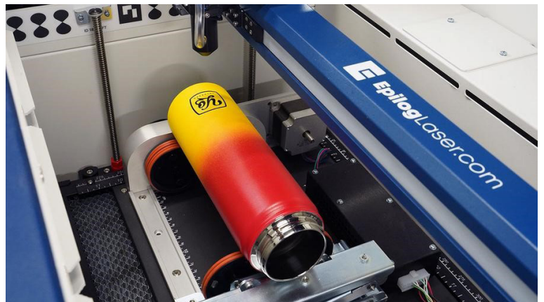
Figure 2: Epilog's 'rim-style' rotary attachment is an optional accessory that adds the ability to engrave cylindrical items to the Fusion Edge line. Source: Epilog Laser
