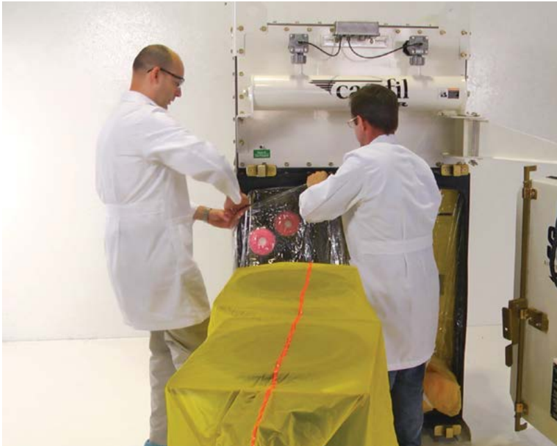
Operators perform a bag-in/bag-out (BIBO) filter change designed to simulate real-world operating conditions.
