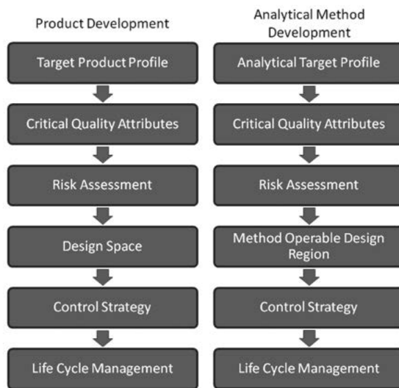
Figure 1: QbD workflows for product development and the analogous workflow for analytical method development.
