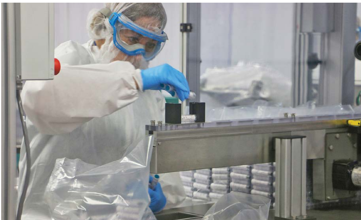
Workers load auto-injector device components into the machine which takes the drug supplied in an ampule and assembles it into the pen.
