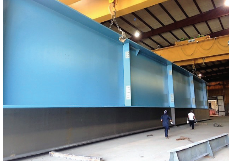
Coating the majority of steel offsite in shop conditions helped to ensure efficient, accurate applications that kept the project on schedule.
