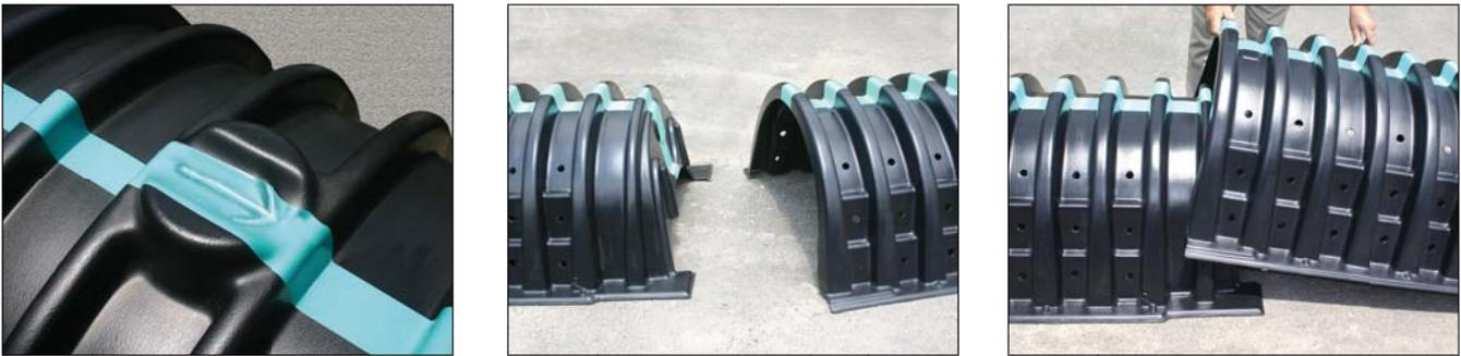
*Directional arrows located on the top of the chamber point towards the Small Rib End. The open end of the next chamber overlaps the small rib end of the preceding chamber.*
