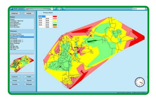
**Asset management** Most utilities burdened with obsolete assets and financial constraints are faced with a "replace or repair" dilemma. Hydraulic models, GIS, CMMS, and other technology tools have proven to be effective in supporting decisions involving predictive versus corrective maintenance (see **Figure 5**). This allows operators to make informed decisions on where and when these actions should be carried out, saving time and money in the process.
