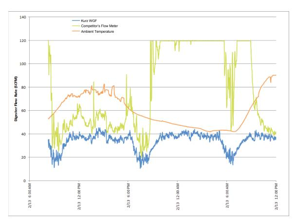
As shown in the graph, when the ambient temperature is cool (in this case, evening and early morning), the original competitor's flow meter reports false high readings and takes some time to respond to digester changes in cooler weather. As the outside temperatures rise, the readings from the competitor's flow meter began to agree with the Kurz WGF.
