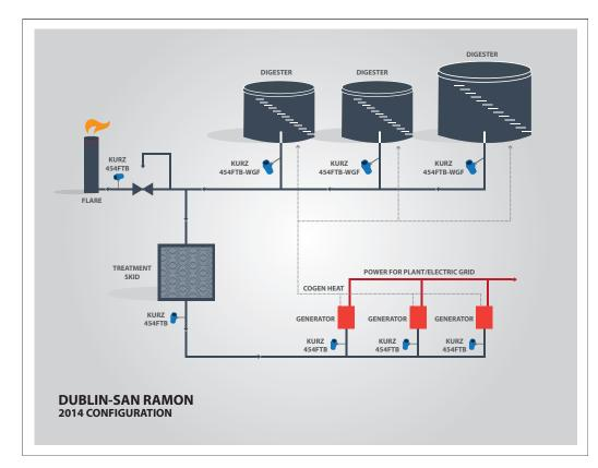
Prior to the installation of the Kurz meters biogas flow measurements remained erratic. The measurements for treated dry gas only matched overall biogas production during the heat of the day. The relationship of temperature changes, especially colder weather, affecting condensation levels and flow measurements was not fully understood at the time.
