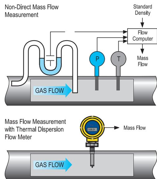
Figure 2. Thermal Mass Flow Versus Other Flow Technologies
